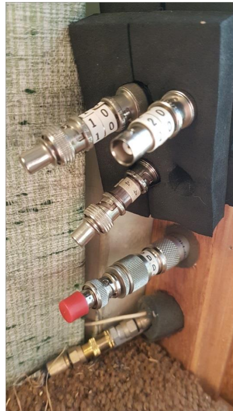
Inside terminated & shorted lines disconnected from all radios
