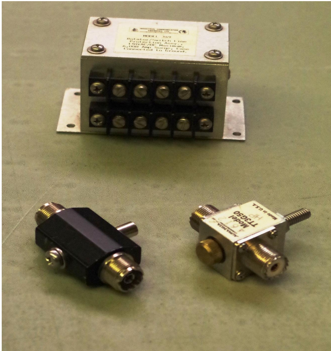
Figure 1 Top: Rotator arrestor (4 pole); Bottom: Various coax arrestors
